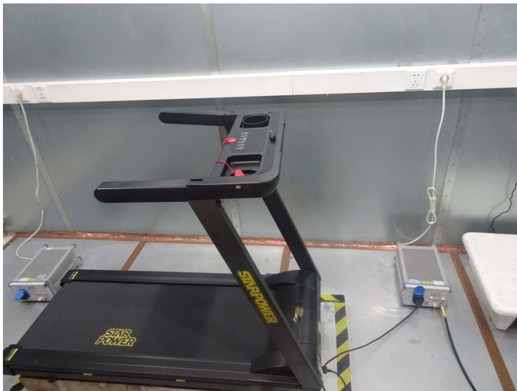
Picture 2: Conducted Emissions Test Setup
