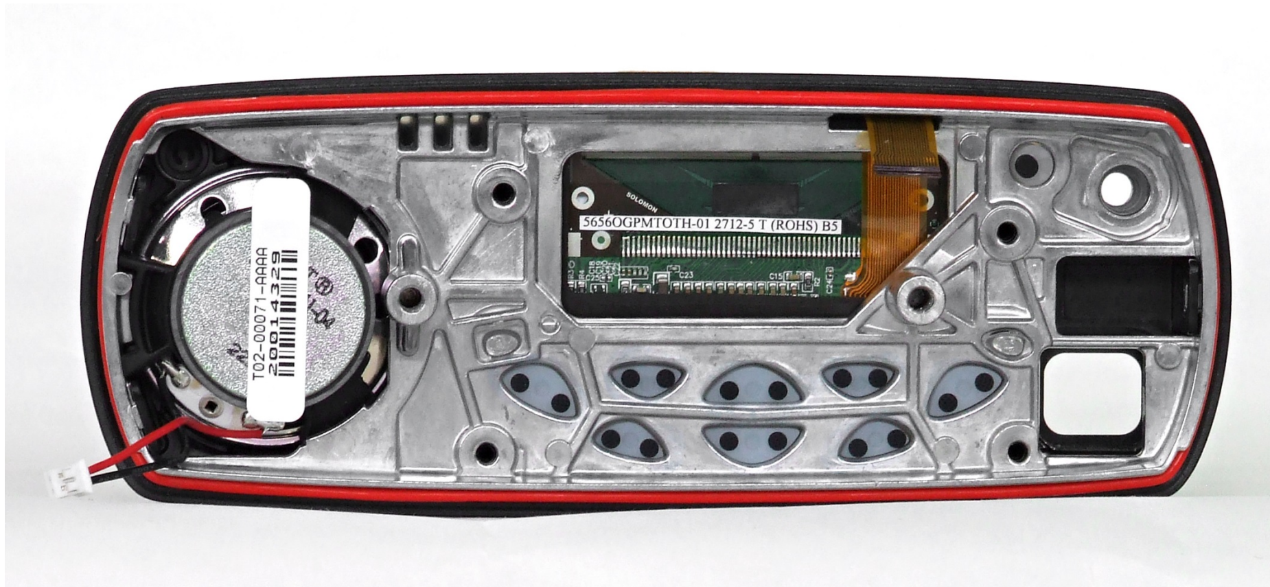
Photograph 06: Control Head – Internal with main PCB removed
