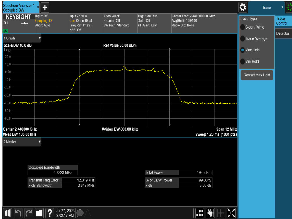
Plot 7-11. 6dB BW & 99% OBW Plot (Bluetooth (HDRp8), 8Mbps – Ch. 37)
