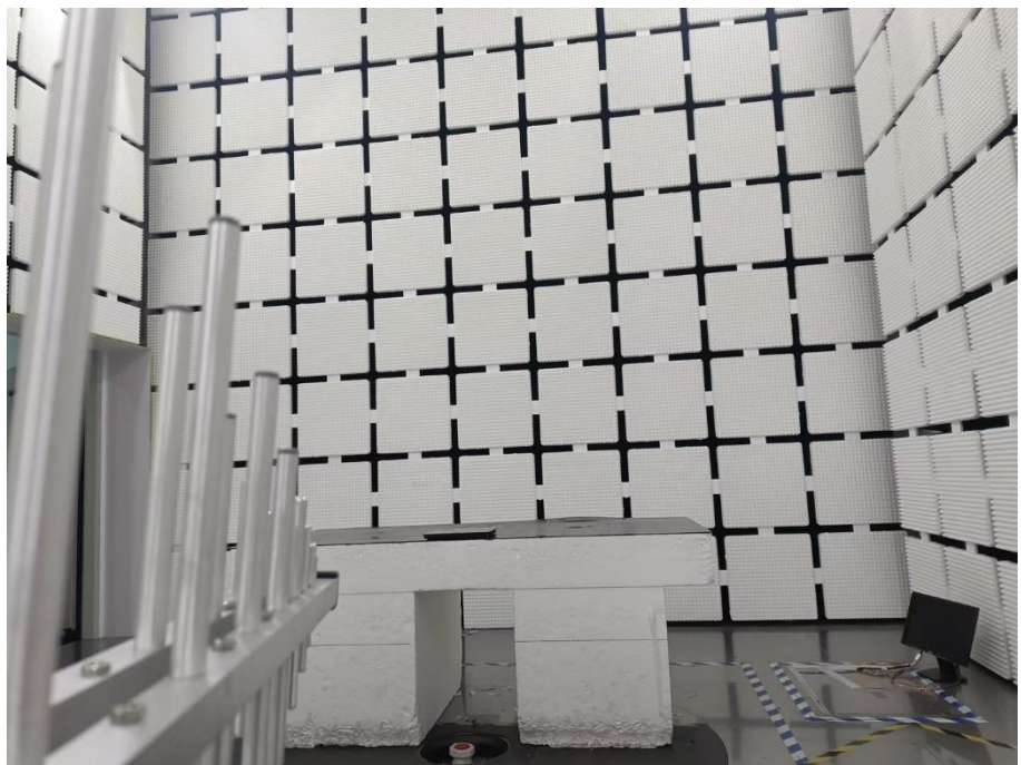
Radiation Emission Test Setup (30MHz to 1GHz)
