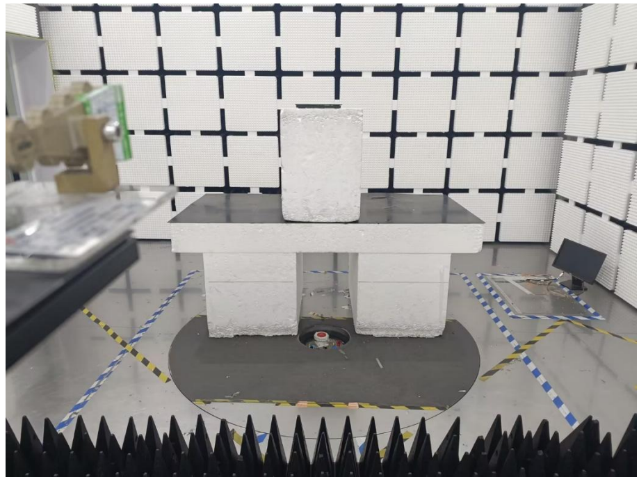
Radiation Emission Test Setup (Above 18GHz)
