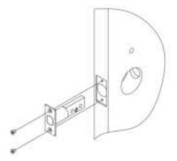
5.Install the front plate and back plate as the diagram, the cylinder trail of the front plate need be horizontal.
