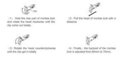
4. When you install the mortise lock, please keep the latch retracted for left to outside or right to inside direction. For the right to outside or left to inside direction please adjust the latch to release with screwdriver.
