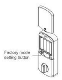
If you forget the master code, you can remove the battery cover and Insert one pin to the factory mode setting button. Keep pressing it for 3sec until one "DING" sound, the system would be reset and all data would be cleared.
