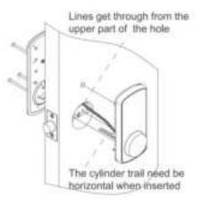
6. Combine the lines to the plug on the back plate, then install the back plate on the back pad. Please fasten the extra lines to the back pad rather than stuff the lines to the holes.
