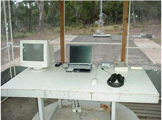
Radiated Emissions Test Setup (10 metre test distance)
