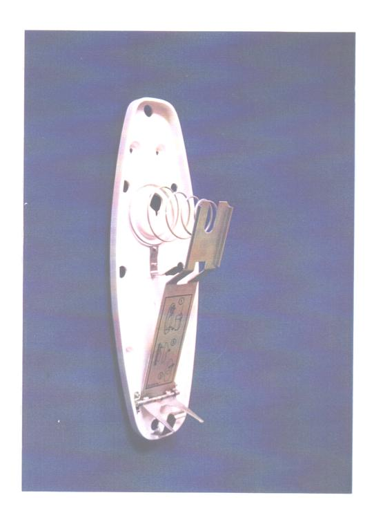
Float Free Enclosure with HRU and retaining rod removed
