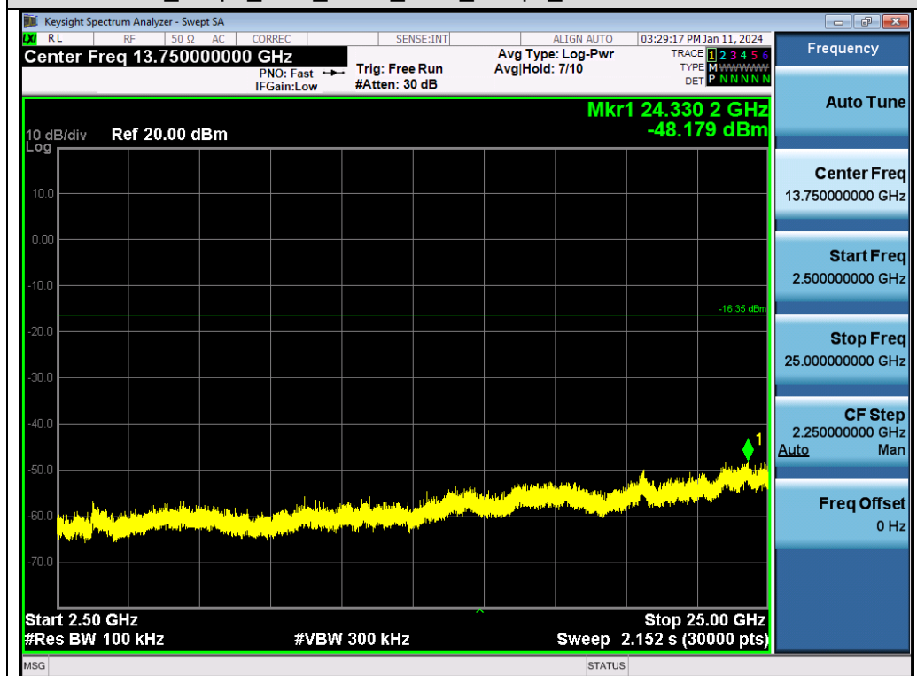
Test_Graph_EDR_ANT1_2480_2Mbps_Higher Band Emissions
