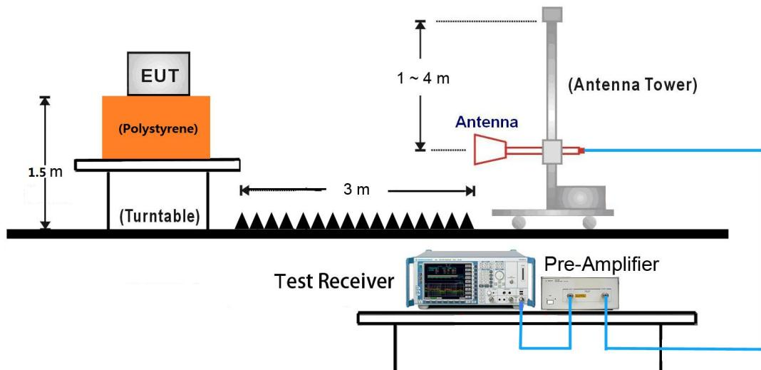
18GHz ~25GHz Test Setup:
