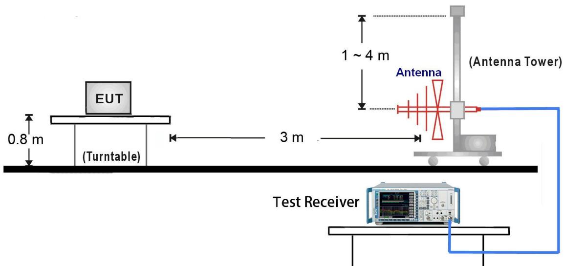
1GHz ~ 18GHz Test Setup:
