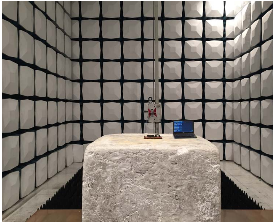
Description: Radiated Emission Test Setup for 1~18GHz
