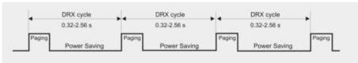
Figure 30: Power saving and paging in LTE networks
