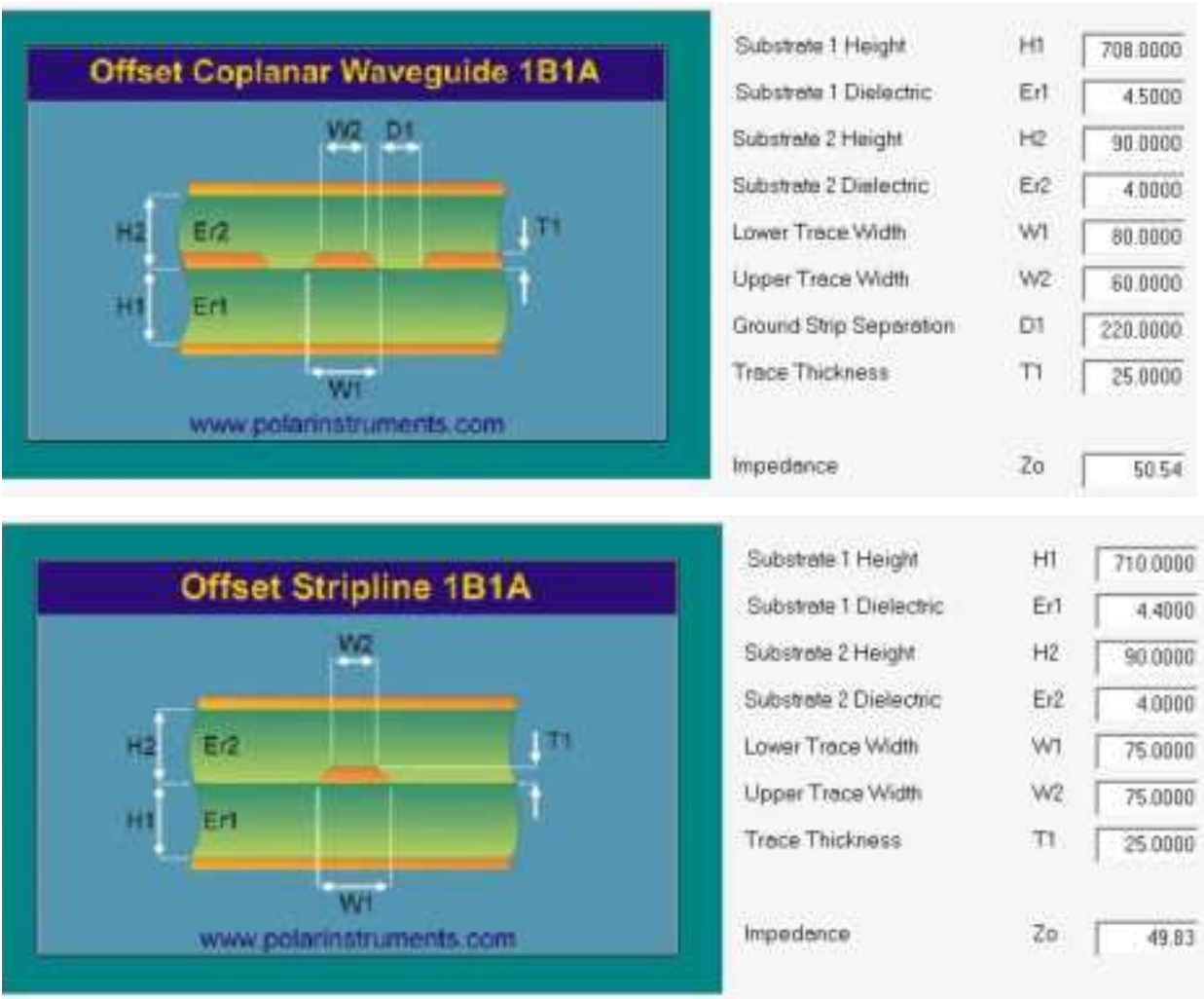
Figure 19: Embedded stripline arrangement example
