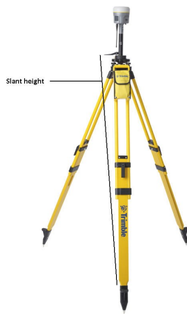
Receiver tripod and tribrach setup with an internal 450 MHz Tx radio (Measuring Slant Height)
