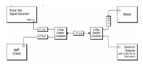
The radio was set at the center channel frequency of tested Channel. A FCC approved mater device – (FCC ID: Q87-WBV-AP230) AP was used to link with the UUT (Client) device.
