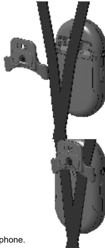
**When attaching a neck strap to the microphone, hook each side of the strap to each claw, and reverse the above procedure.**
