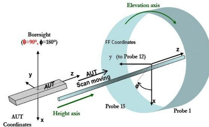
Coordinate system – Spherical geometry
