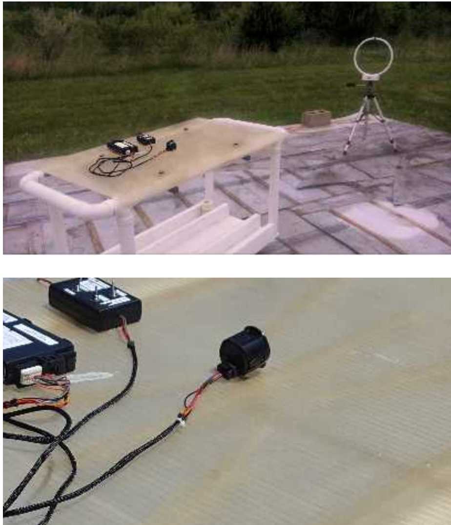
Figure 4: Radiated Emissions Test Setup Photograph(s).
