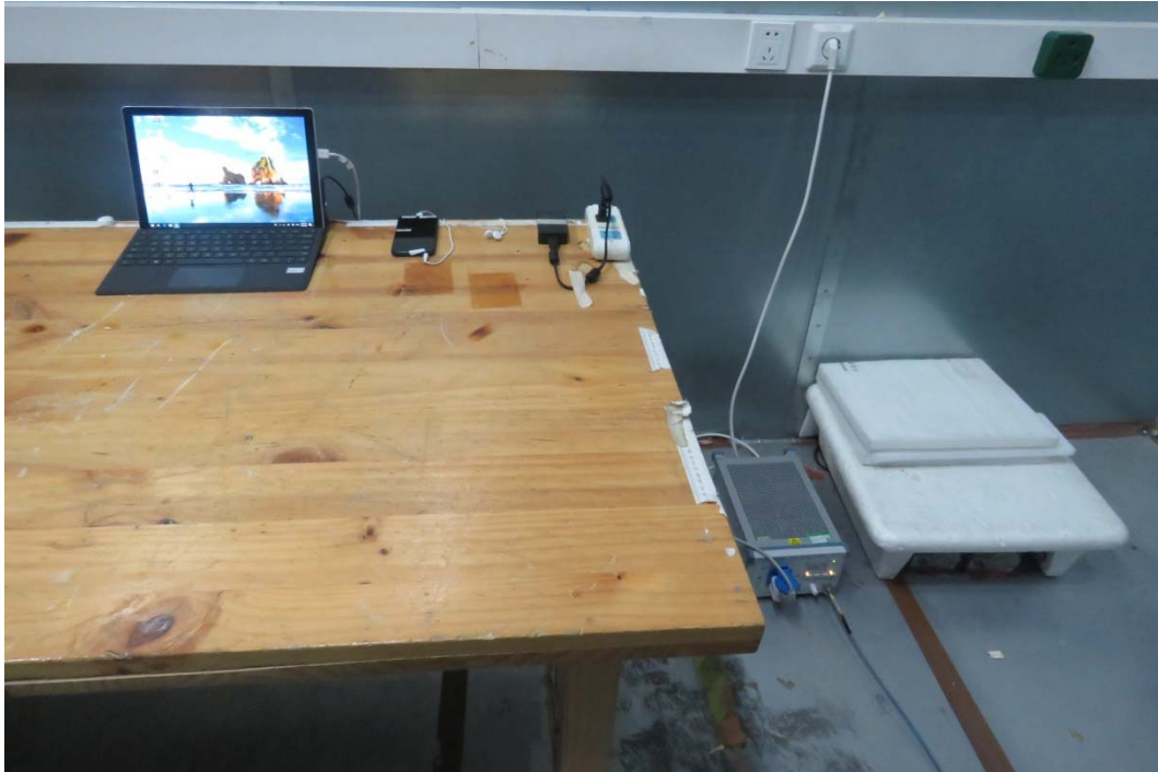
Picture 2 Conducted Emission Test Setup
