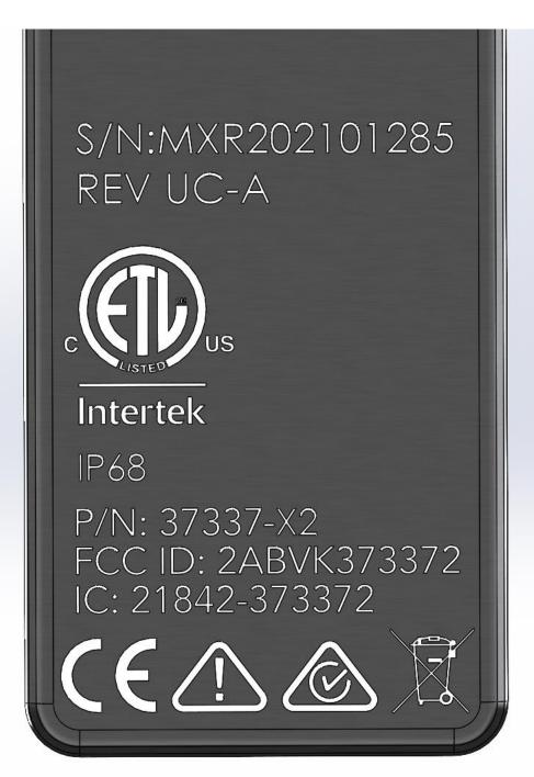
The Label is laser etched onto the back of the EUT. The label measures 2 cm wide by 2.5 cm tall
