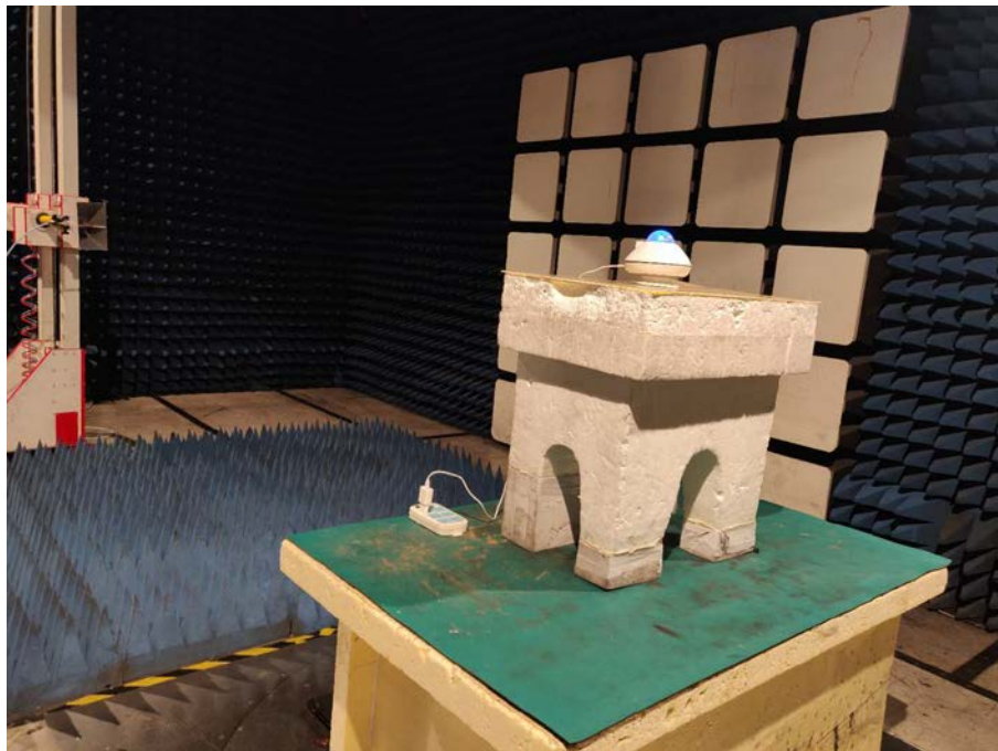
Spurious Emission Test Setup (Above 1GHz)
