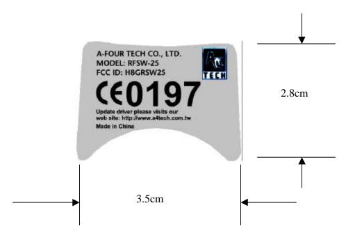
The remained portion of lable statement required by FCC is attached in the user's manual.
