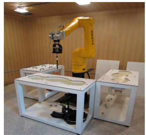
Figure E.7.1 DASY5 Test System
