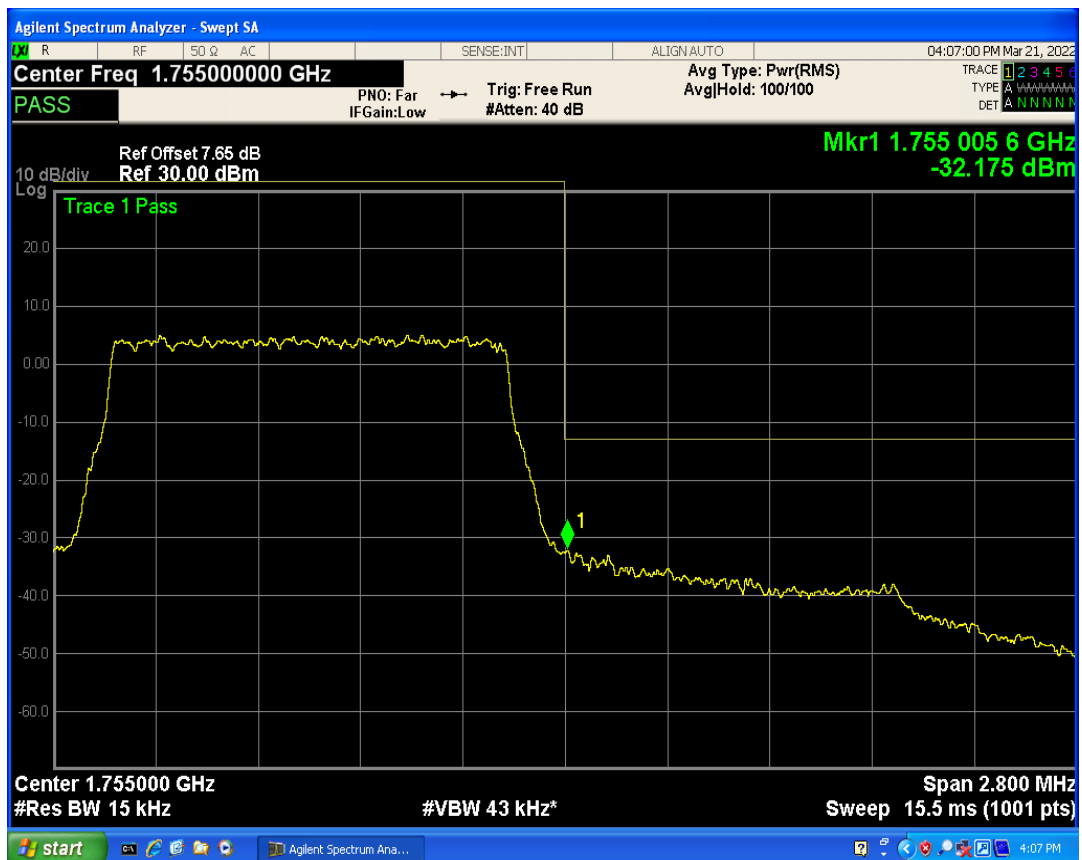
Band4 QAM16 BW=1.4MHz Channel=20393 RB Size=1 Position=#0
