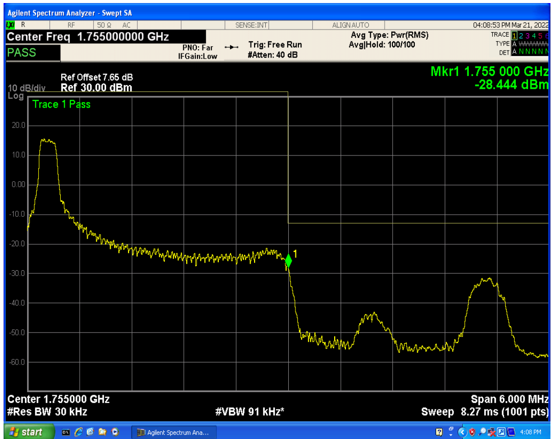
Band4 QAM16 BW=3MHz Channel=20385 RB Size=1 Position=#Max
