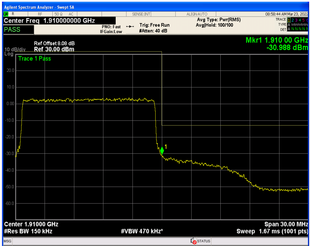
Band2 QPSK BW=20MHz Channel=18700 RB Size=1 Position=#Max
