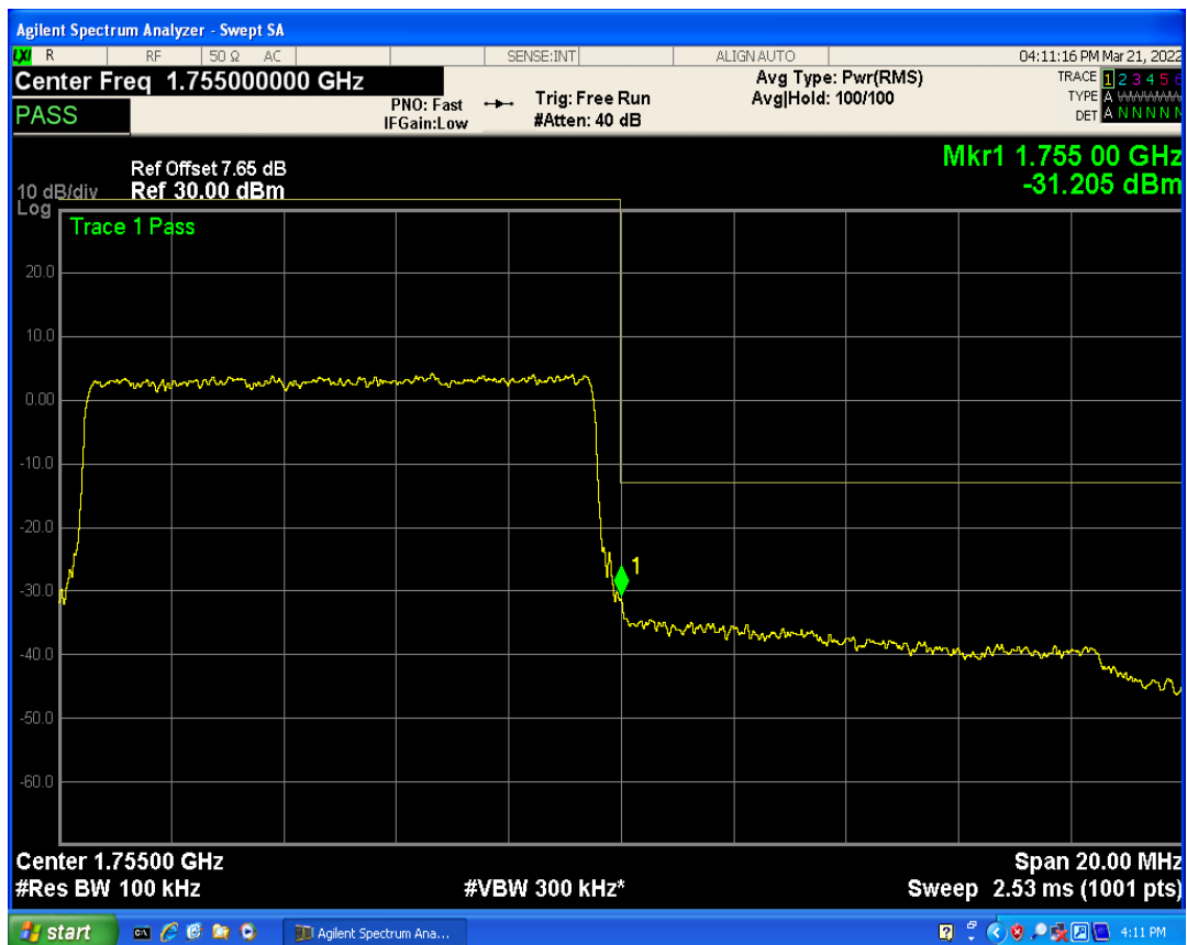
Band4 QAM16 BW=10MHz Channel=20350 RB Size=1 Position=#0
