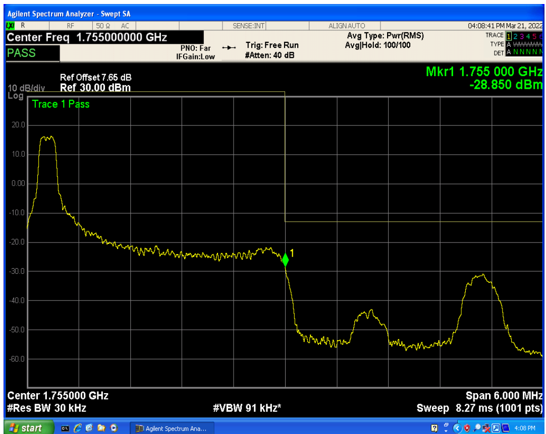
Band4 QPSK BW=3MHz Channel=20385 RB Size=15 Position=#0
