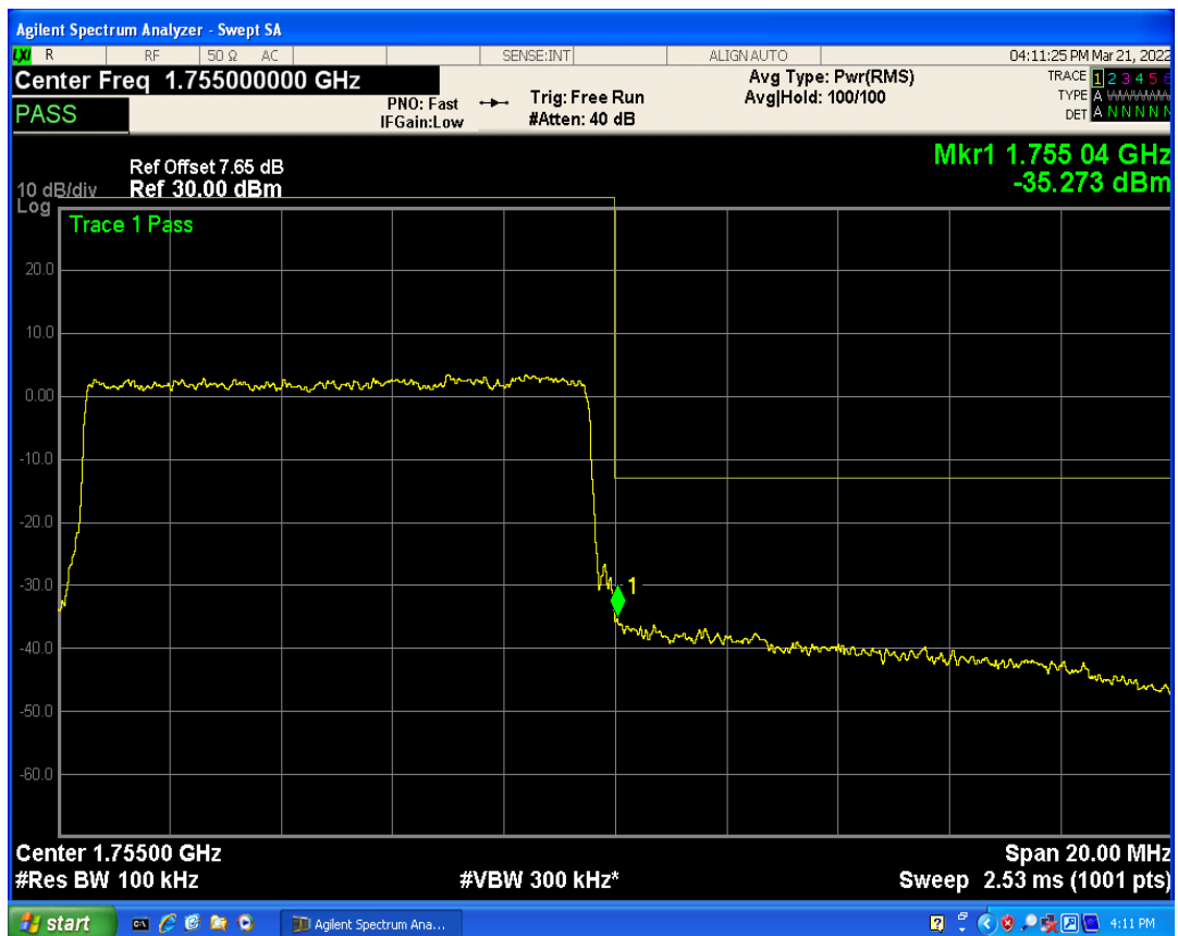
Band4 QAM16 BW=10MHz Channel=20350 RB Size=1 Position=#Max
