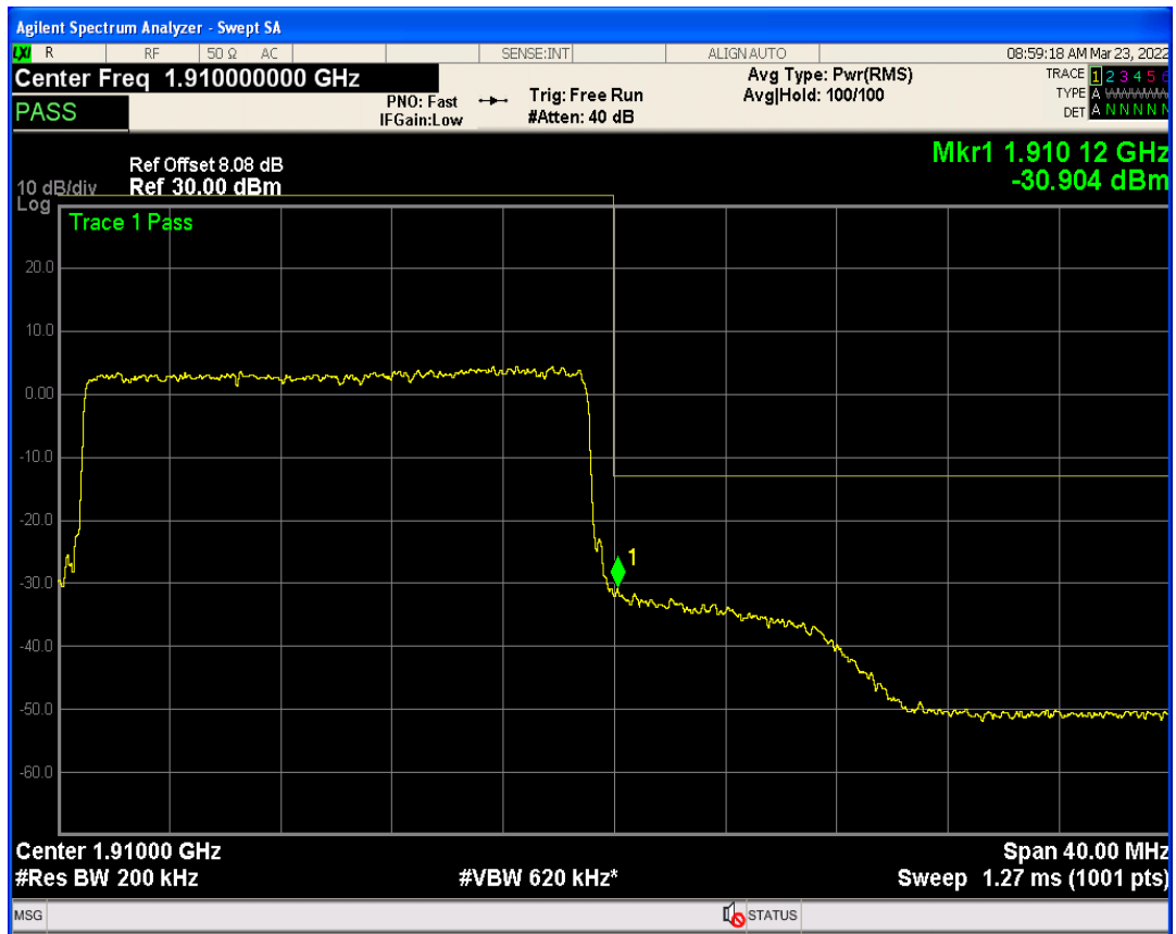
Band2 QAM16 BW=20MHz Channel=19100 RB Size=1 Position=#Max
