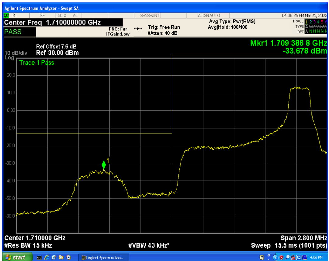
Band4 QPSK BW=1.4MHz Channel=19957 RB Size=1 Position=#0
