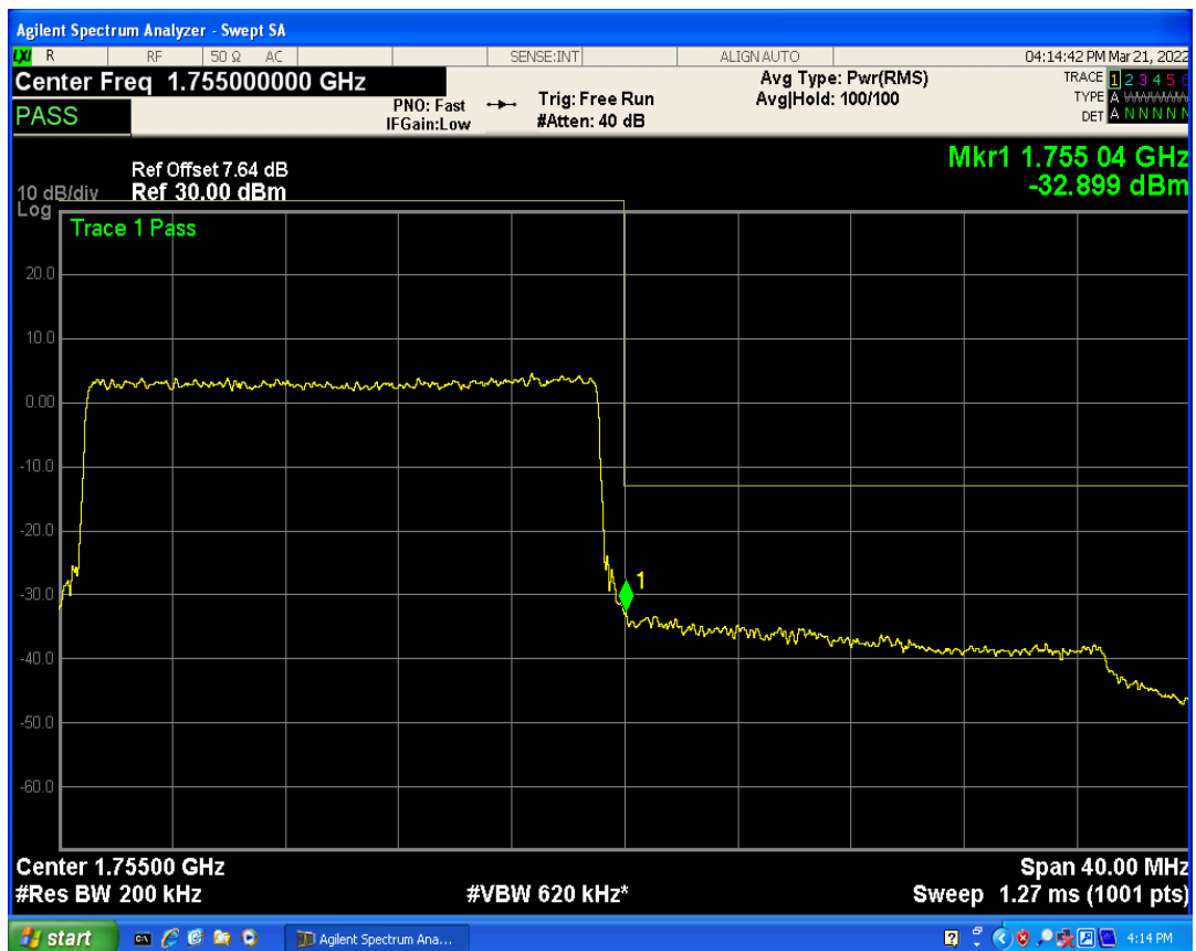
Band4 QAM16 BW=20MHz Channel=20300 RB Size=1 Position=#0
