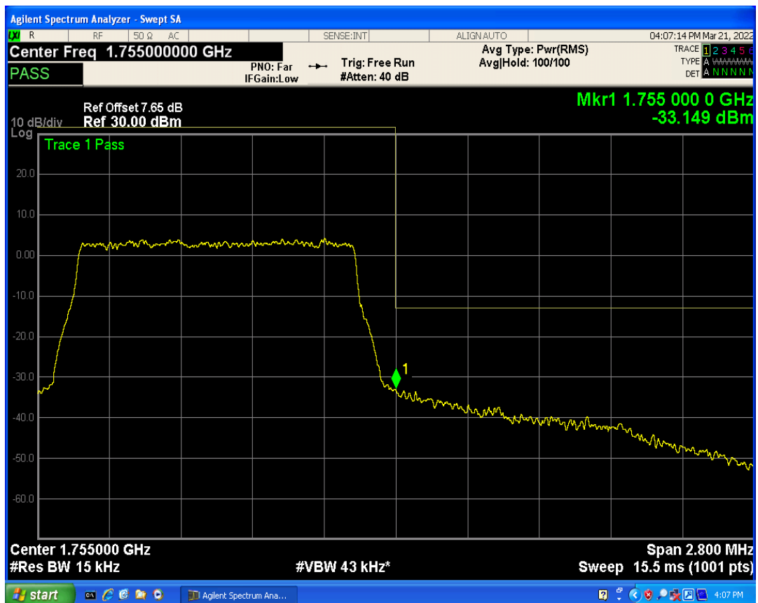
Band4 QAM16 BW=1.4MHz Channel=20393 RB Size=1 Position=#Max
