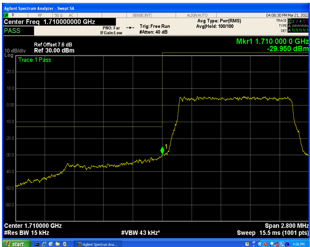
Band4 QAM16 BW=1.4MHz Channel=19957 RB Size=1 Position=#0
