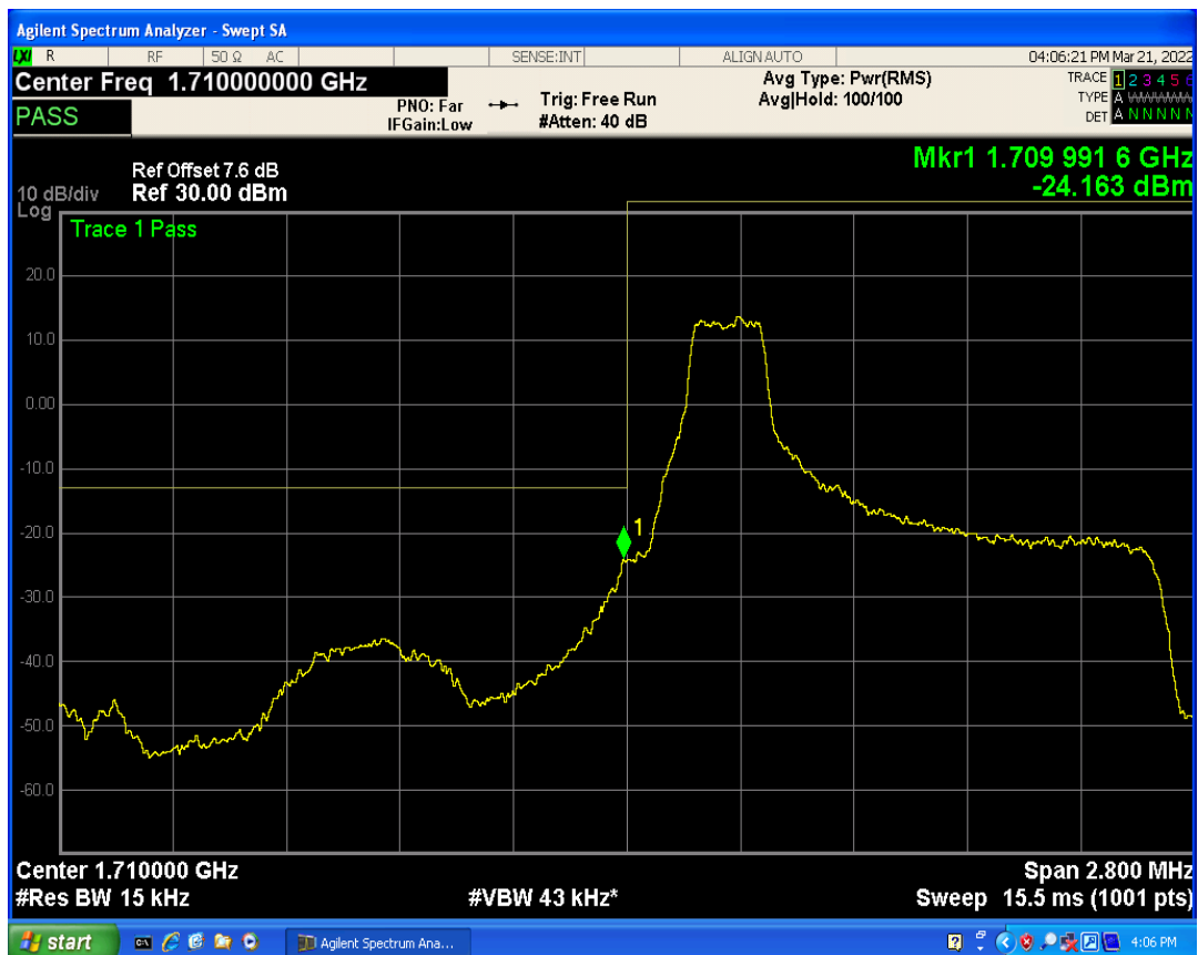
Band4 QPSK BW=1.4MHz Channel=19957 RB Size=6 Position=#0
