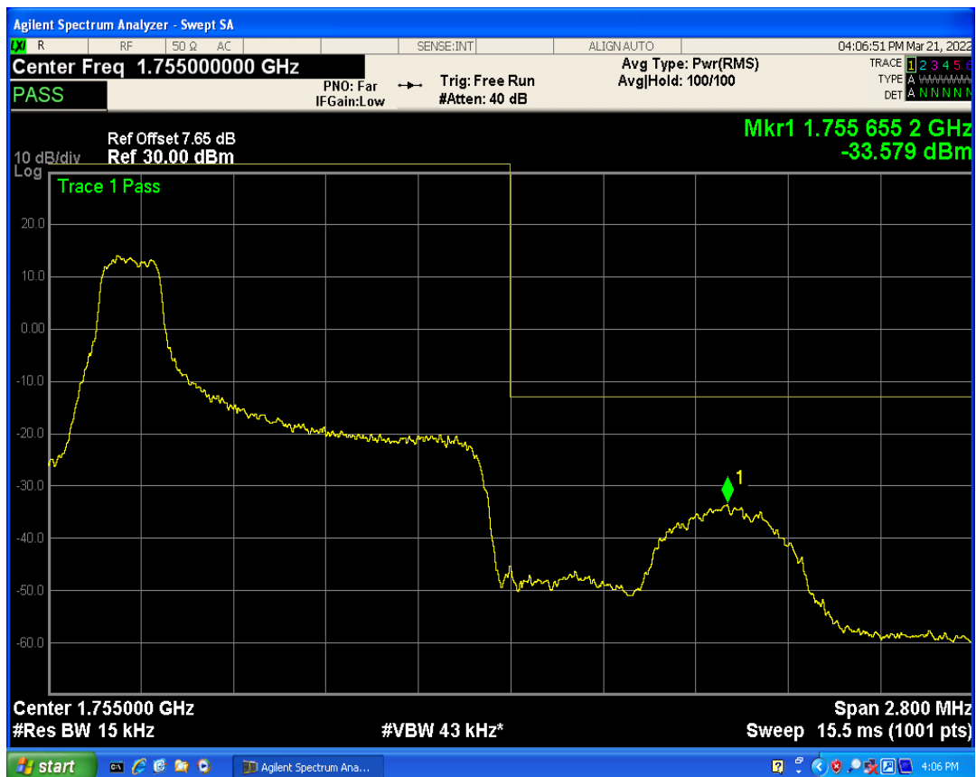
Band4 QPSK BW=1.4MHz Channel=20393 RB Size=1 Position=#Max
