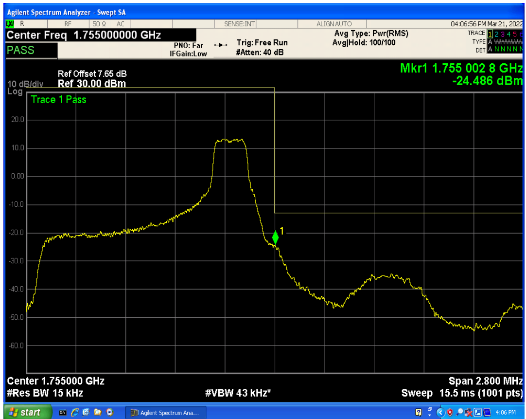
Band4 QPSK BW=1.4MHz Channel=20393 RB Size=6 Position=#0
