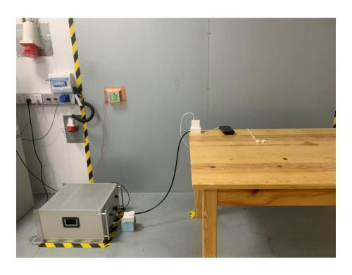
Set-up for Radiated Emission (RE), Below 1GHz
