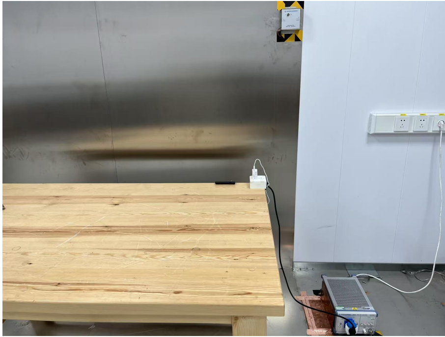
Radiated Emission Test View|(Below 1G)
