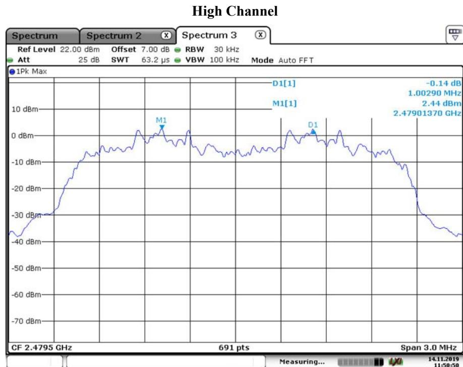
**FCC §15.247(a) (1)–BANDWIDTH TESTING****Applicable Standard**
