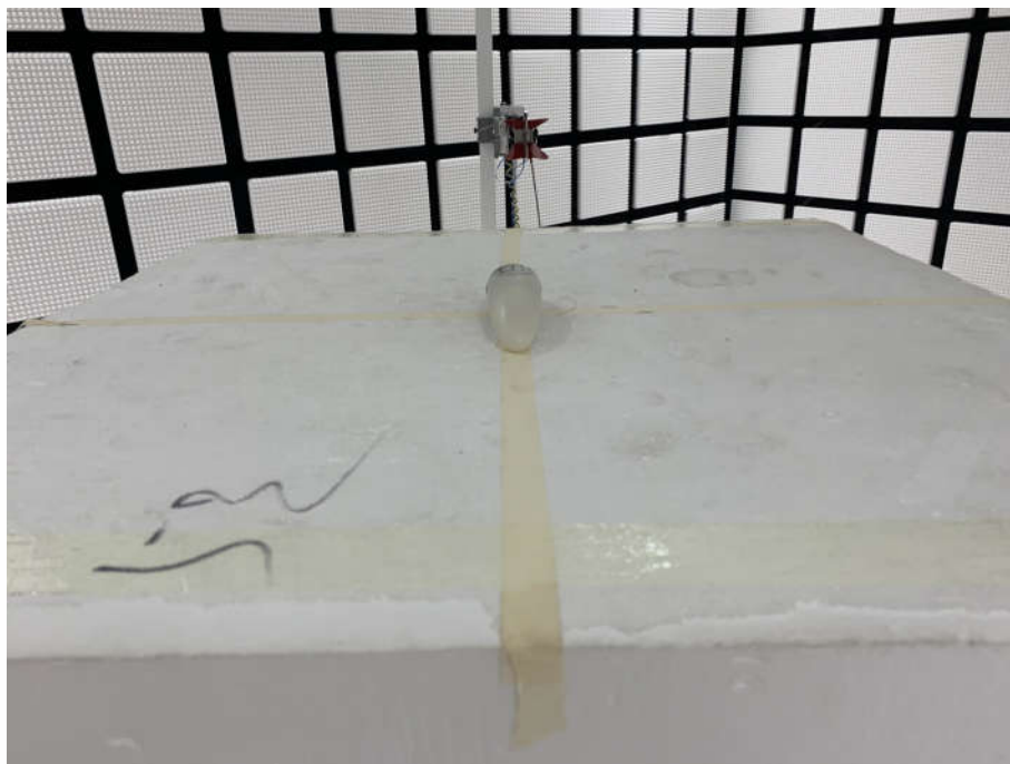
Radiated spurious emission Test Setup-2(Above 1GHz)
