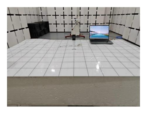
Set-up for Radiated Spurious Emission, Above 1GHz
