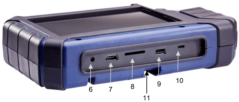
Fig. 7: Bottom side of the monitor with USB and SD card slot
