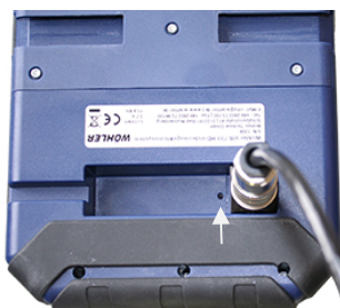
Fig. 51: Reset hole indicated by an arrow
