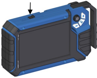
Fig. 14: Push button for pulling out the handle marked with arrow
