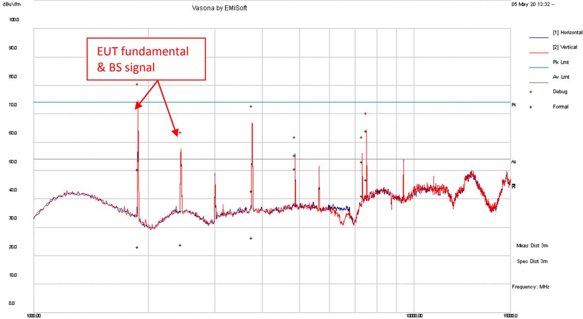
Radiated Emissions Template: FCC 15.209 (3m) 1GHz-18GHz
