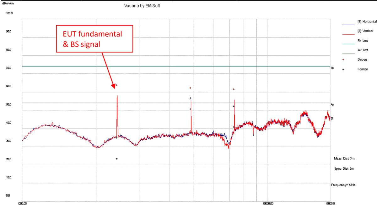
Radiated Emissions Template: FCC 15.209 (3m) 1GHz-18GHz
