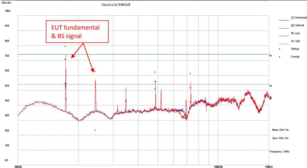
Radiated Emissions Template: FCC 15.209 (3m) 1GHz-18GHz
