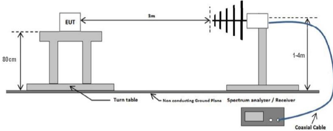
Radiated emissions test setup above 1 GHz
