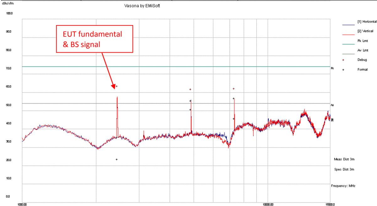
Radiated Emissions Template: FCC 15.209 (3m) 1GHz-18GHz
