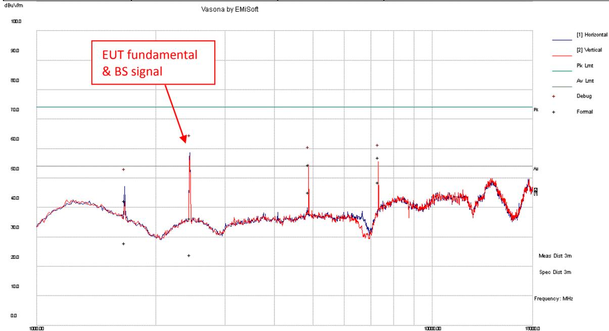
Radiated Emissions Template: FCC 15.209 (3m) 1GHz-18GHz
