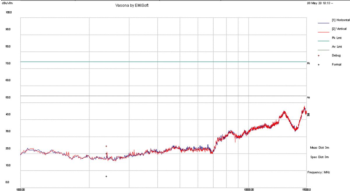
Radiated Emissions Template: FCC 15.209 (3m) 1GHz-18GHz
