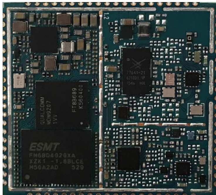
EUT- Top Shielding Cover off Zoom View (EC25-A)
