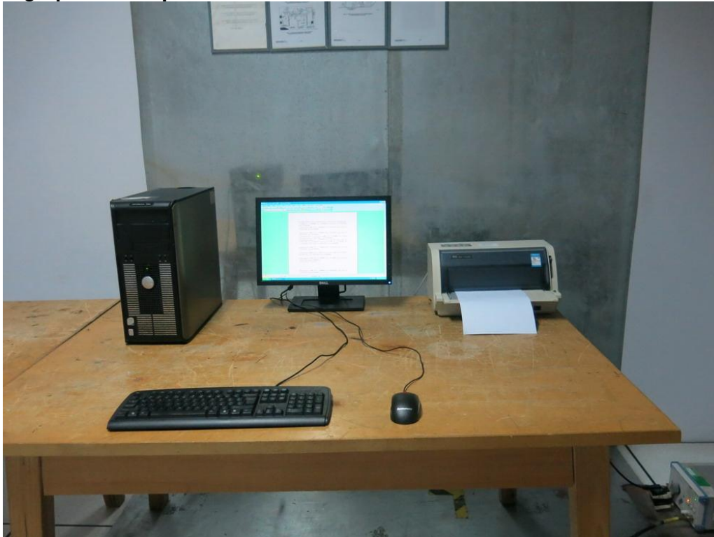
Photograph 2: Set-up for Radiated Emissions of below 1GHz
