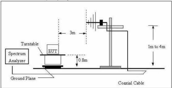
(C) Radiated Emission Test-Up Frequency Above 1GHz
