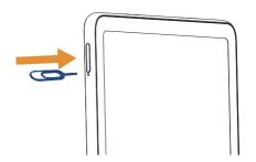
Step 2. Remove the NANO SIM card/microSD card tray.
