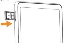
**Step 4.** Slide the tray slowly into the SIM tray slot. It only fits one direction. Do not force into place. Keep the SIM tool in a safe place for future use.
