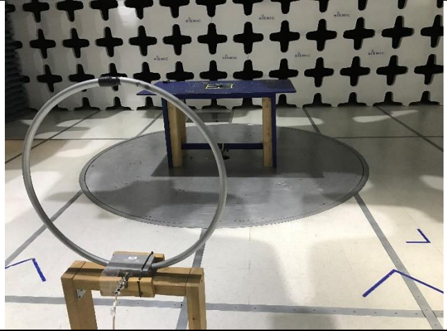
Radiated Emissions (<30MHz) – Rear View
