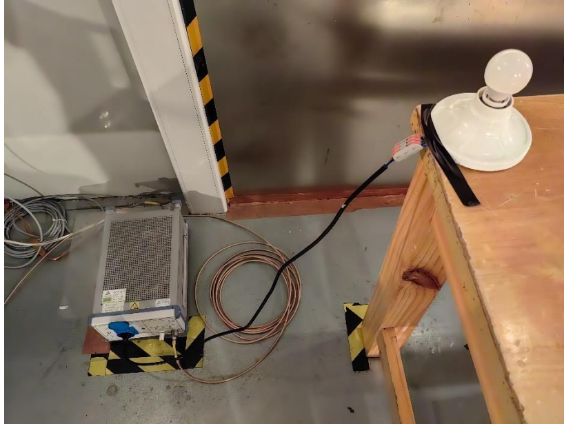
Photograph 2: Set-up for measurement of radiated emission
