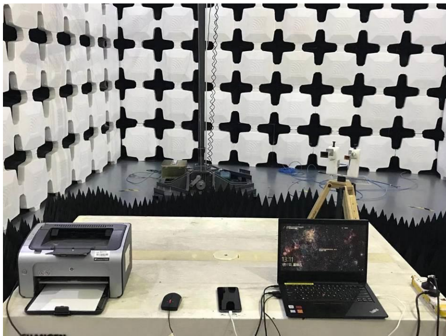
4. Radiated Emissions (Part 15B,Data transfer Mode) (26.5GHz-30GHz)
