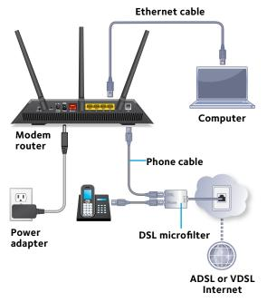
You can use a wired connection to connect a computer to the modem router, or you can use a WiFi connection to connect a computer or WiFi device to the modem router:
