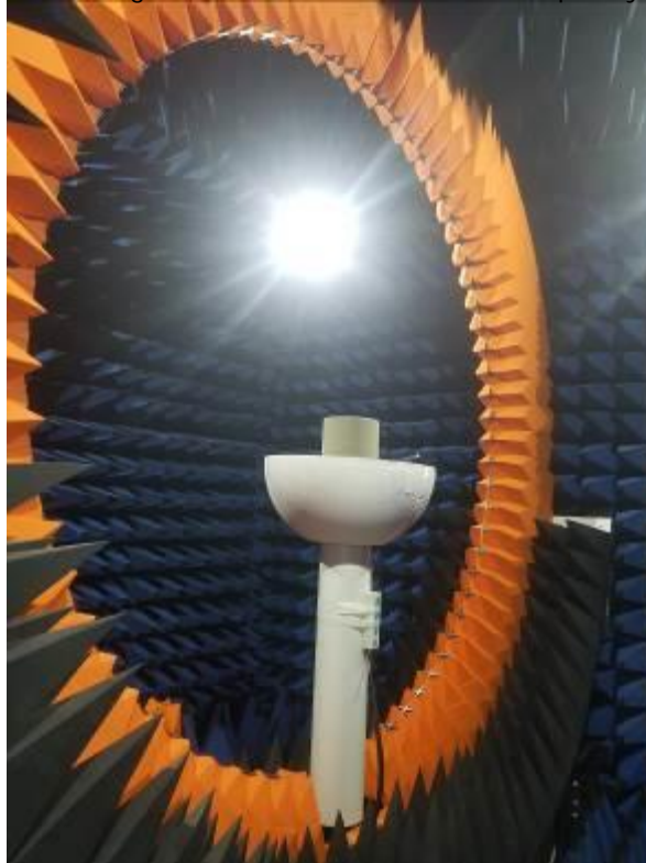
Fig. 4 Satimo anechoic chamber test system
