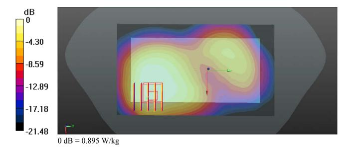
Communication System: UID 0, LTE (0); Frequency: 707.5 MHz; Duty Cycle: 1:1
