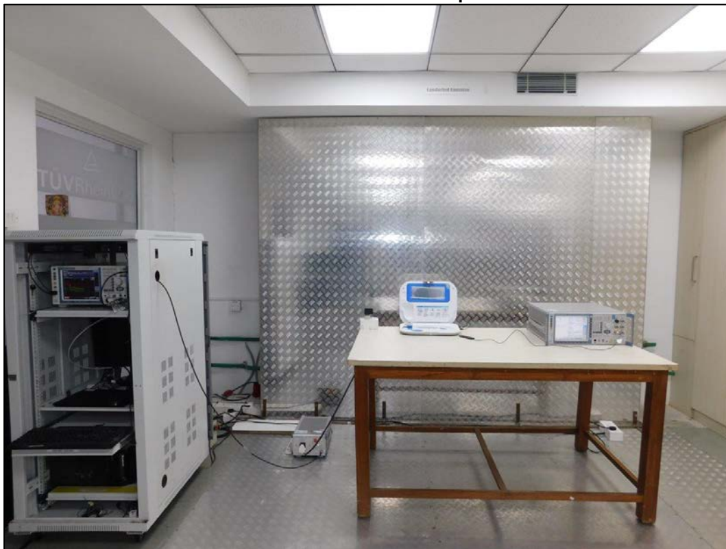
Conducted Emission Test
