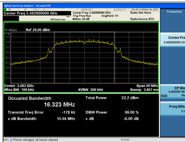
6 dB Bandwidth plot (802.11n_HT20-CH 11)
