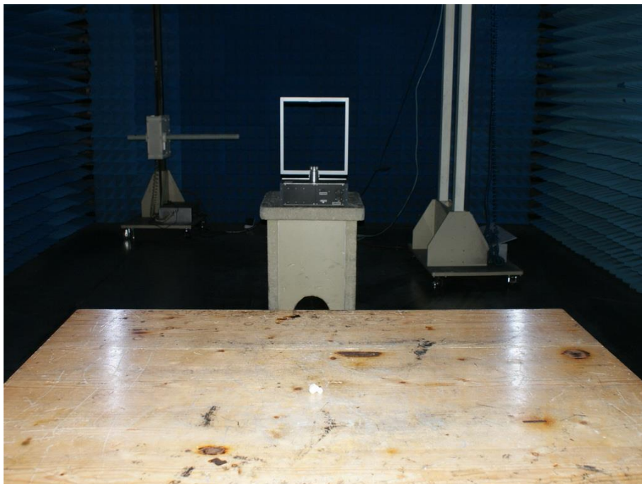
Photograph 4: Set-up for Radiated Spurious Emission, below 30MHz
