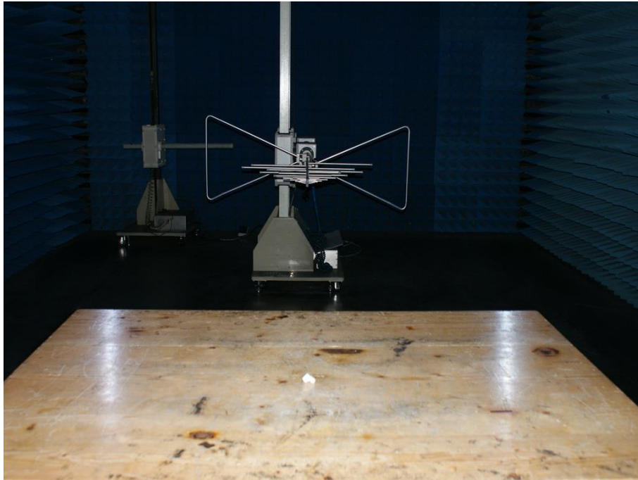
Photograph 5: Set-up for Radiated Spurious Emission, 30MHz - 1GHz
