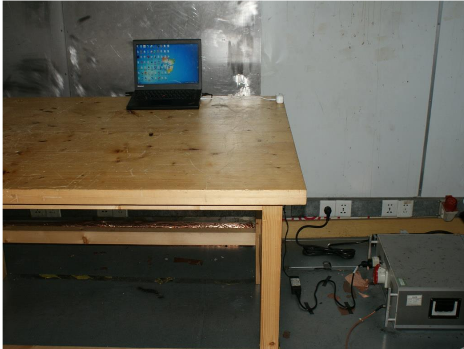
Photograph 1: Set-up for Conducted Emission on AC Mains
