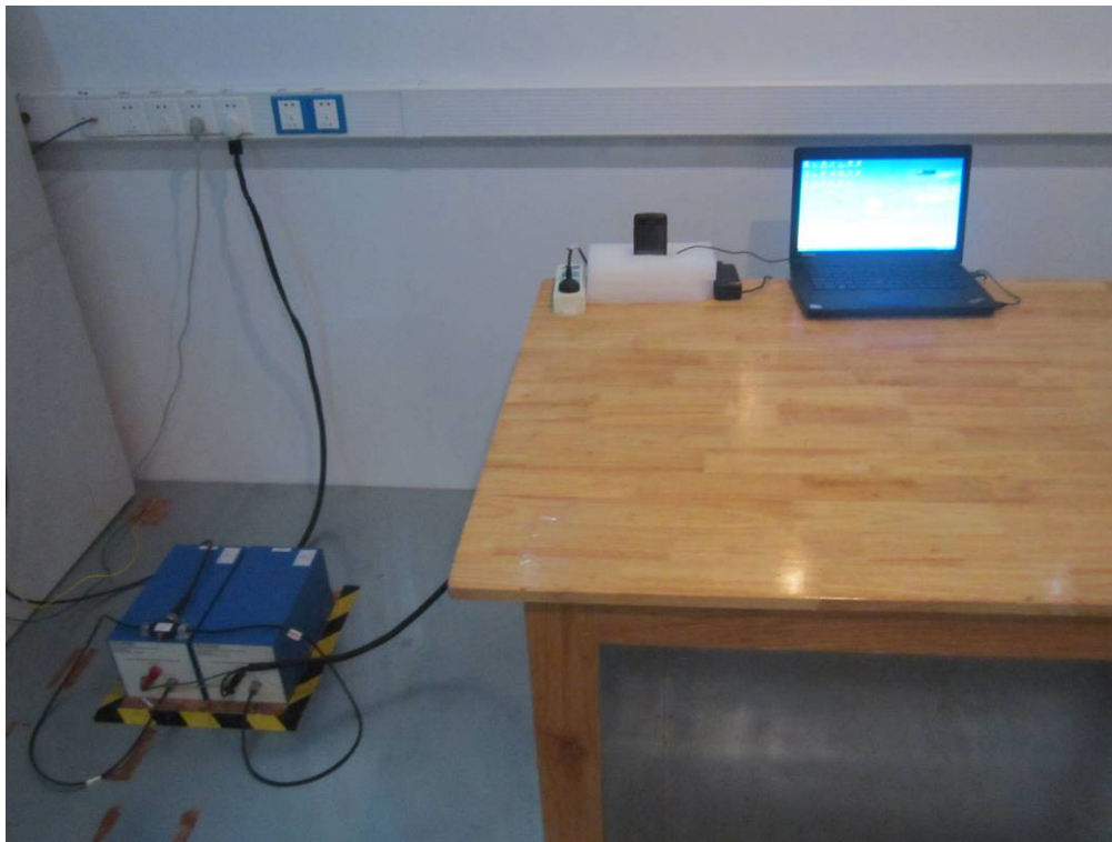
Conducted Emissions Test Setup Front View
