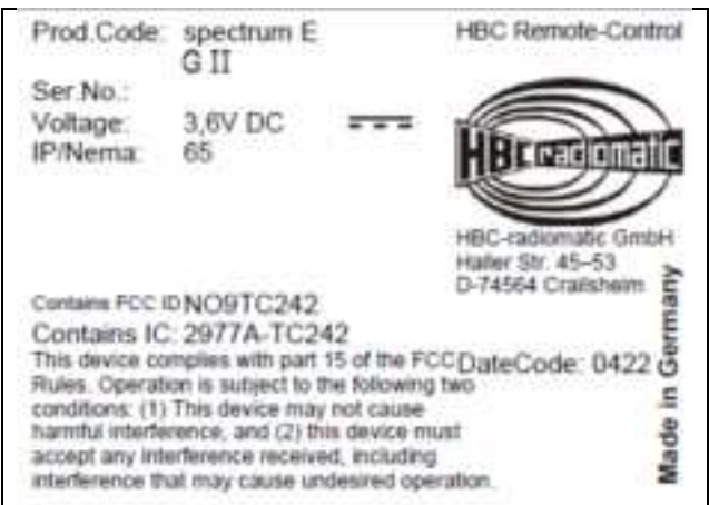
Figure 1: Example type plate of a host device
