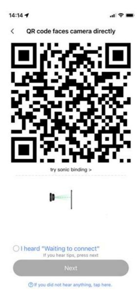
The QR code that appears on the mobile phone is scanned against the camera lens, and the device emits a prompt sound "QR code scan successful" and "WiFi connected", click Next, and wait for the network configuration to be completed.
