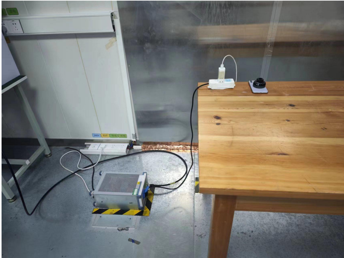
Conducted emission test setup
