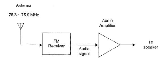
The RF signal from the transmitter is received through the antenna. The signal is then downconverted and demodulated by the FM receiver IC. The audio signal is amplified and fed into the speakers to get the acoustic signal.
