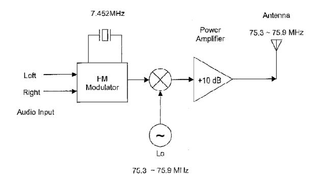
Analog signals are inputed into the FM Modulator to form the multiplexed FM signal and then upconverted to 75.3 ~ 75.9 MHz. The RF signal is then amplified by a power amplifier and radiated through the internal antenna
