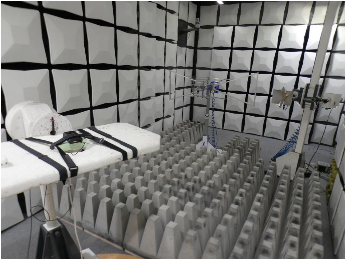
Photo 1: Test setup with EUT C for radiated emissions measurements above 1 GHz in the fully anechoic room (FAR)
