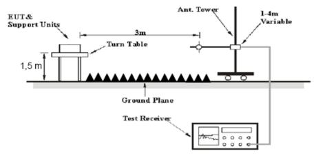
The radiated emission below 1GHz tests were performed in the 10 meters chamber, above 1GHz tests were performed in the 3 meters chamber B, using the setup accordance with the ANSI C63.10-2013. The specification used was the FCC 15.209, and FCC 15.247 limits.
