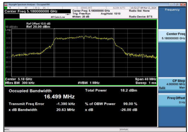
U-NII-1 99% & 26dB Bandwidth-802.11a(20MHz) ,5180MHz,Ant1
