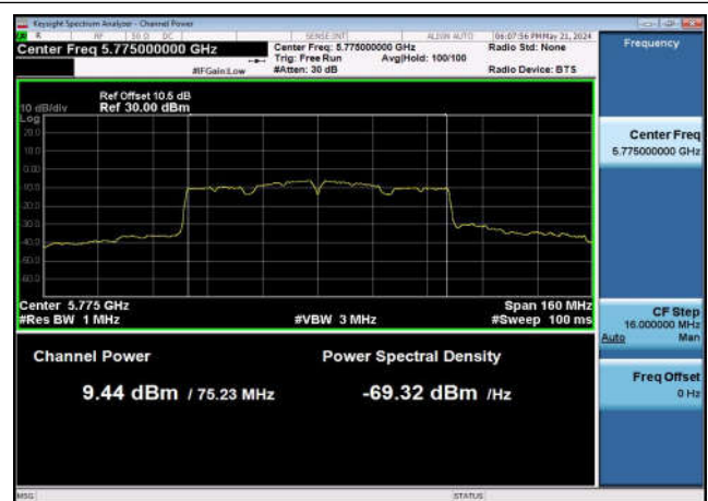
U-NII-3 Output Power-802.11ac(80MHz) ,5775MHz,Ant1
