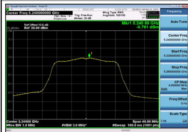
U-NII-1 Power spectral density-802.11 ac(20MHz),5240MHz,Ant1
