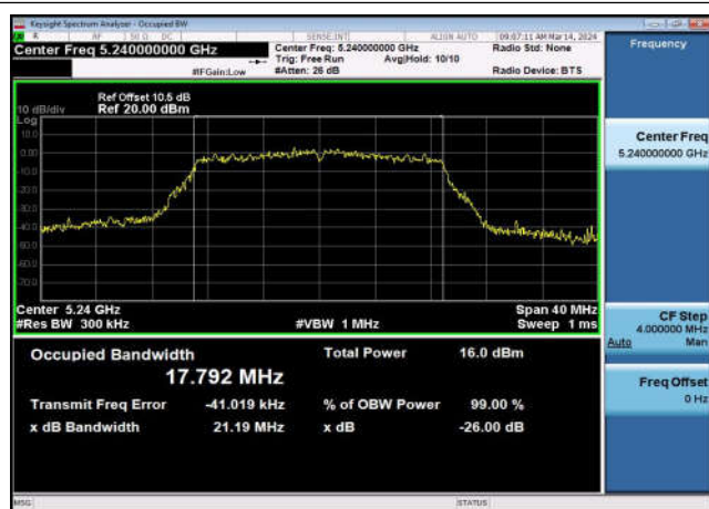
U-NII-1 99% & 26dB Bandwidth-802.11ac(20MHz) ,5240MHz,Ant1
