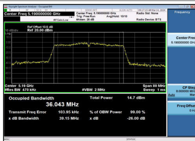
U-NII-1 99% & 26dB Bandwidth-802.11ac(40MHz) ,5190MHz,Ant1
