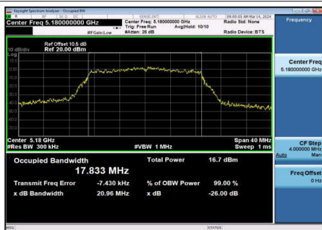
U-NII-1 99% & 26dB Bandwidth-802.11ac(20MHz) ,5240MHz,Ant1
