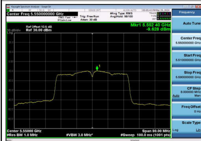
U-NII-2c Power spectral density-802.1 1a(20MHz),5500MHz,Ant1
