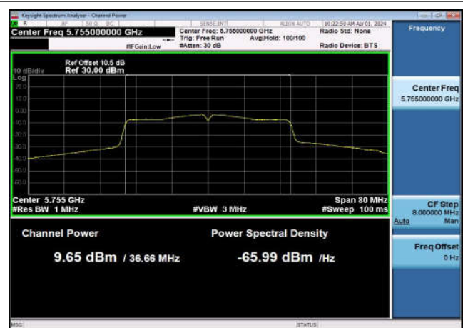
U-NII-3 Output Power-802.11ac(80MHz) ,5775MHz,Ant1
