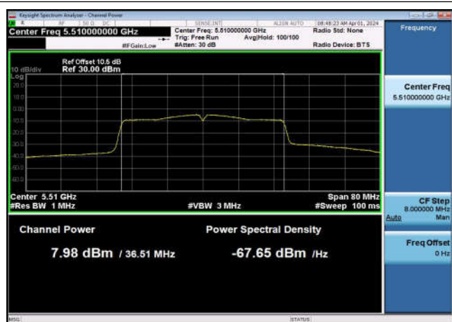
U-NII-2c Output Power-802.11ac(40MHz) ,5510MHz,Ant1
