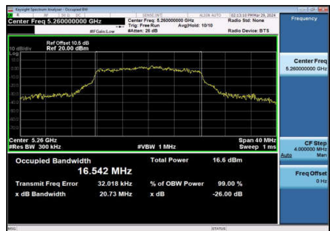
U-NII-2a 99% & 26dB Bandwidth-802.11a(20MHz) ,5320MHz,Ant1
