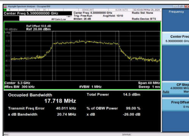
U-NII-2a 99% & 26dB Bandwidth-802.11n(40MHz) ,5270MHz,Ant1
