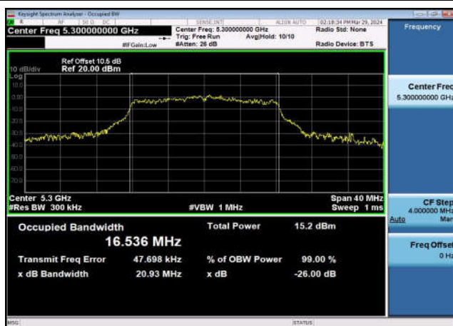
U-NII-2a 99% & 26dB Bandwidth-802.11ac(20MHz) ,5260MHz,Ant1
