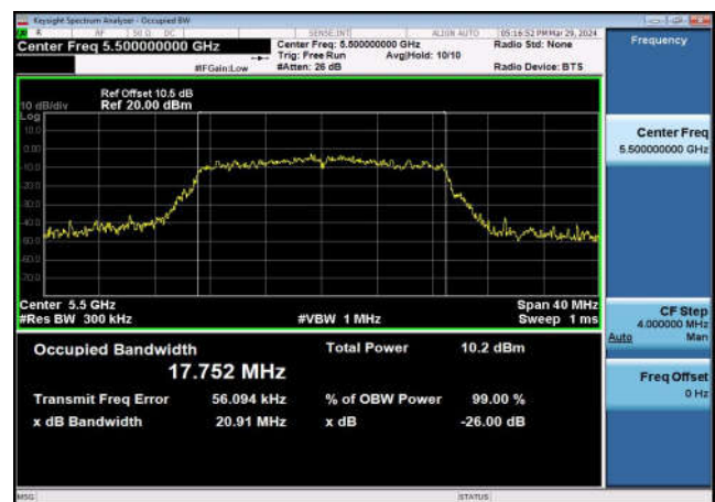
U-NII-2c 99% & 26dB Bandwidth-802.11ac(20MHz) ,5700MHz,Ant1
