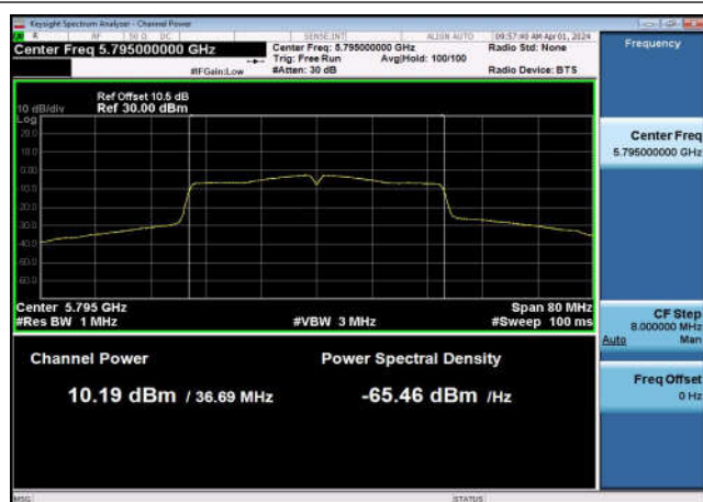
U-NII-3 Output Power-802.11a(20MHz) ,5785MHz,Ant1
