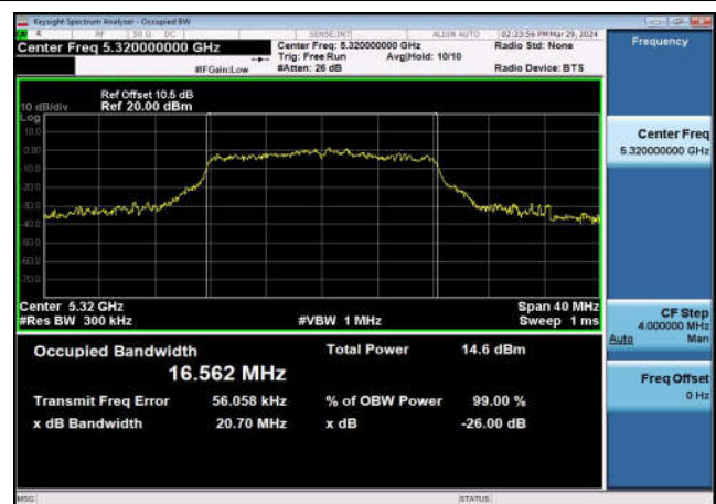
U-NII-2a 99% & 26dB Bandwidth-802.11ac(20MHz) ,5300MHz,Ant1
