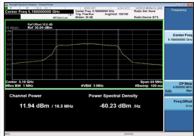
U-NII-1 Output Power-802.11a(20MHz) ,5180MHz,Ant1
